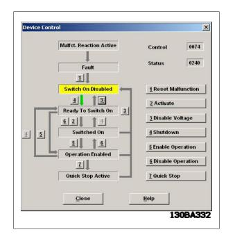
Click 4 for Ready to Switch On and click 2 for Switch On. Upon clicking 5 the VLT frequency converter should start the motor. The control word is now 7F Hex. Press Close.
